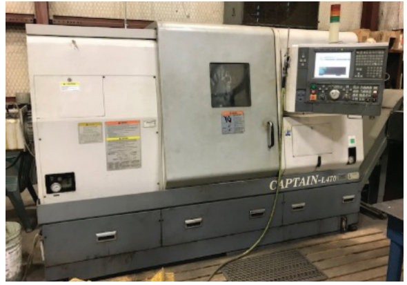
Okuma Lathe – 15" dia x 24" long
