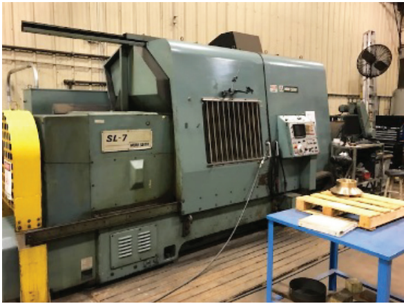
Mori Seiki – SL7 Lathe – 24" x 4" long
