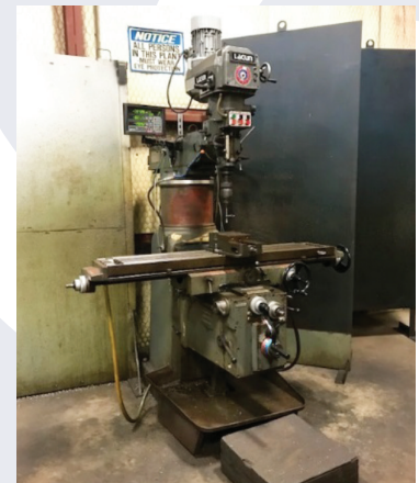
Bridgeport mill 12" width x 5' length
