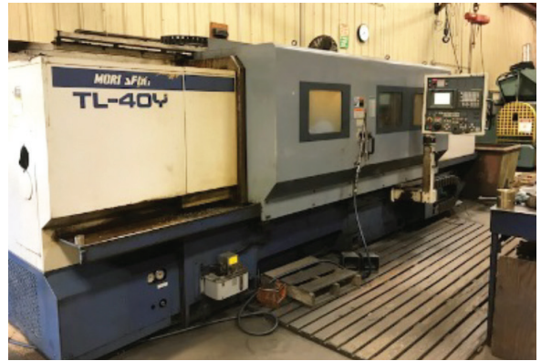
Mori Seiki – TL40Y Turning Center 18" diameter x 10' long, Live Tooling, Y axis
