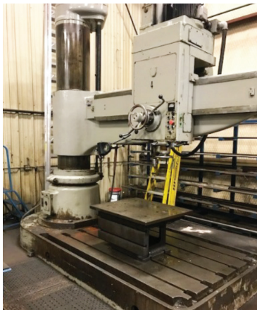
Radial drill press 16" column x 6' arm
